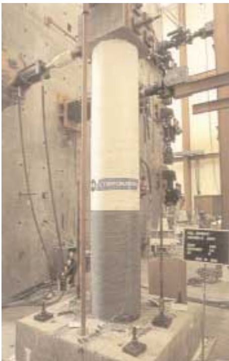
Column test installation for California Department of Transportation.
