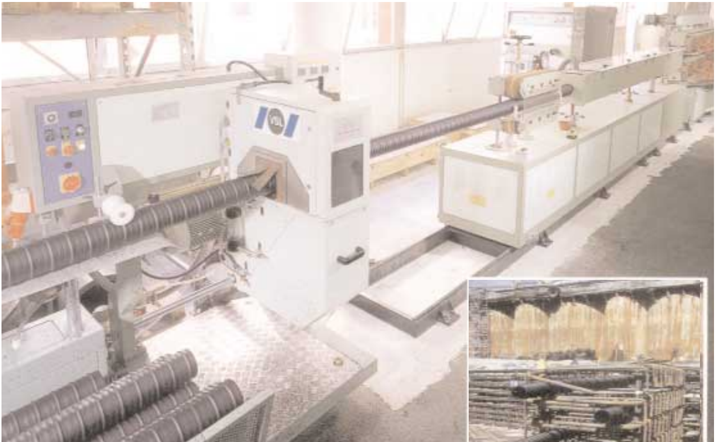
Above: Manufacturing of VSL PT-PLUS Plastic Duct. Right: PT-PLUS Plastic Duct will be installed in the TROLL North Sea offshore platform. TROLL is the tallest Condeep platform ever built.
