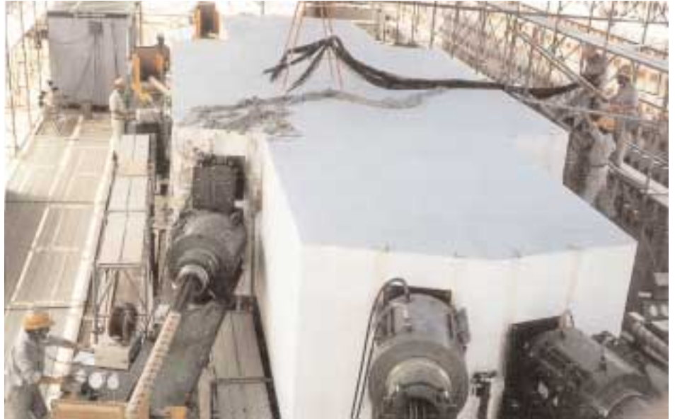
Full scale model test up to a load of 1,060t
